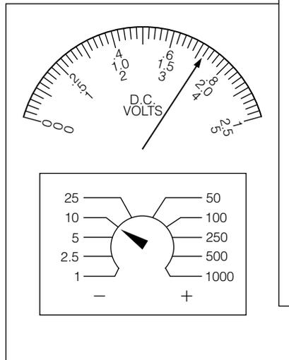
**Figure 5A** This voltmeter has a dial that changes the scale.
