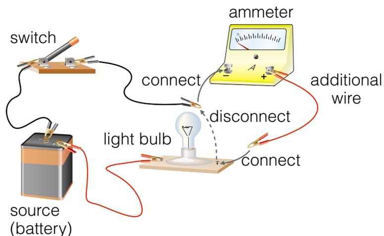
**Figure 2** Connecting an ammeter to a circuit.
