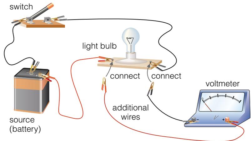
**Figure 3** Connecting a voltmeter to a circuit
