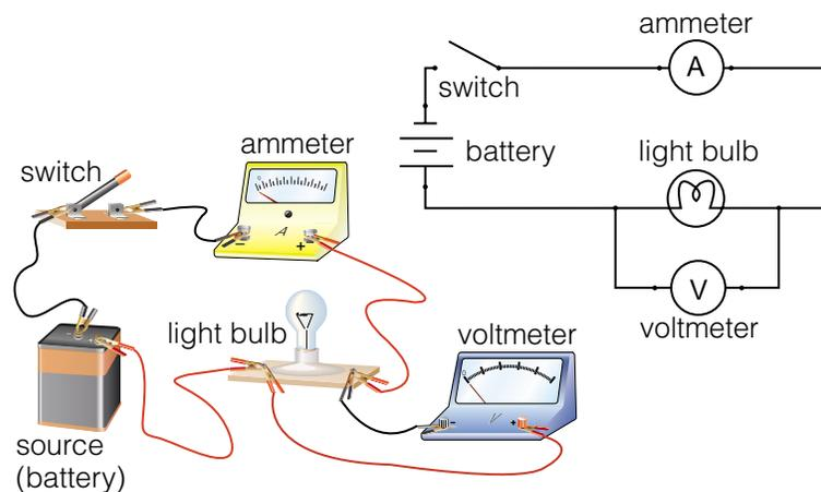
**Figure 1** To measure the current flowing through the light bulb, the ammeter must be connected in series with the light bulb. To measure the potential difference across the light bulb, the voltmeter must be connected in parallel with the light bulb.
