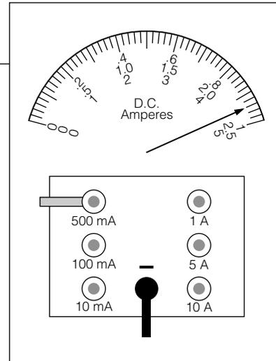
**Figure 5B** This ammeter has different positions in which to plug the positive lead.
