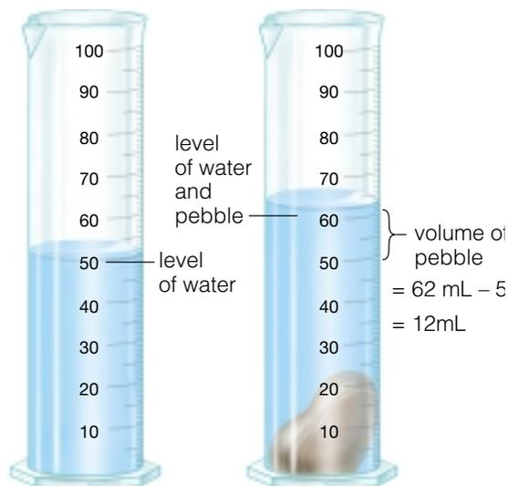
The volume of larger objects can be determined by displacement as well, by using an overflow can. The spout allows water displaced by an object to be caught and measured in a graduated cylinder, as shown in the two diagrams directly below.
