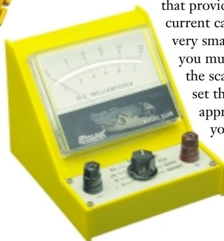
**Figure 4B** Meters that have needles pointing to a dial are called analog meters.
