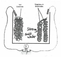
ELECTROCHEMICAL CELL (also called a voltaic cell) (ex. battery):
